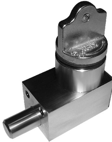
The Type FN interlock has a more narrow housing than the Type F interlock and is mounted by means of 1/4"-20 tapped holes in the end of the housing. All components are constructed from electropolished 316 stainless steel. The lock bolt is 5/8" diameter and the throw, or travel, of the lock bolt is 3/4". Lock bolt movement is completely controlled by the rotation of the key.
